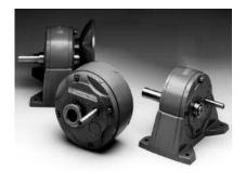
200 Optimount Series helical gear speed reducers contain gears and pinions made of heat-treated alloy steel or close-grain cast iron, with ball or tapered roller bearings. Rugged housings are precisionmachined to assure accurate and permanent gear alignment.
