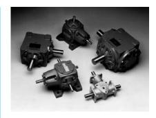
Right-angle gear drives are available with single or double output shafts and are designed for high capacity and efficiency, quiet operation, and long service life. Bevel or spiral bevel gears are made of hardened alloy steel, with oversized bearings and high-quality oil seals.
