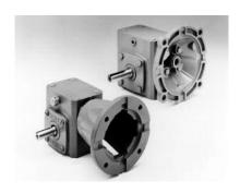
700 Series single-reduction worm gear speed reducers feature integral hardened worms and bronze worm gears. Through-bore housings assure true shaft positioning, proper mating of worm and gear, and perfect alignment under maximum stress conditions. Oversize roller and ball bearings allow greater overhung and thrust loads.
